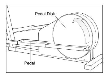
To dismount the elliptical exerciser, allow the pedals to come to a complete stop. **CAUTION:** The elliptical exerciser does not have a freewheel; the pedals will continue to move until the flywheel stops. When the pedals are stationary, step off the highest pedal first. Then, step off the lowest pedal.
